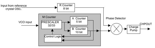
Figure 5. Phase Lock Loop Block Diagram
