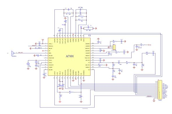
Figure 11. Application Circuit for Transceiver (Data rate = 250Kbps)
